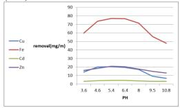
Figure (3): Effect of incubation pH on heavy metals removal
