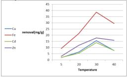
Figure (2): effect of temperature on heavy metals removal
