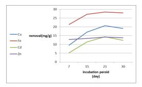
Figure (1): Effect of incubation period on heavy metals removal
